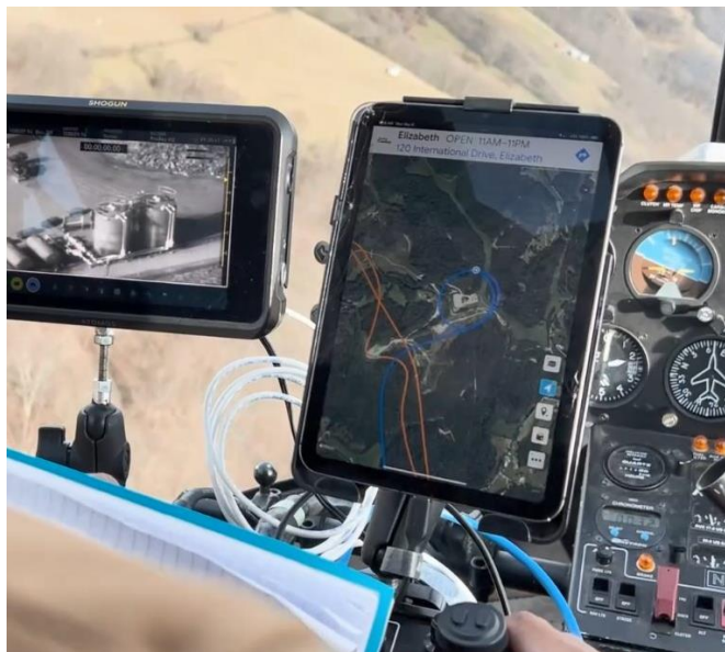
Figure 6. On the left, the screen shows the live OGI image from the camera mounted to the helicopter. On the right, the tablet depicts the helicopter's flight path.
