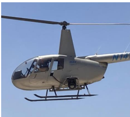
Figure 4. Robinson helicopter (as an example) with an OGI camera and gimbal installed.
