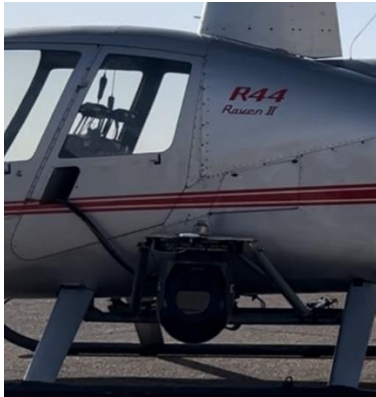
Figure 3. A close shot of the gimbal and OGI camera system installed on a helicopter.
